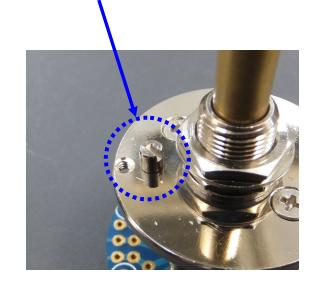
The position can also be changed by turning the mounting plate 180 degrees.
