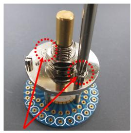
Remove the screws with the phillips head screwdriver. screwdriver.
