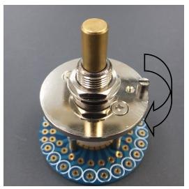
Turn the mounting plate 180 degrees and fix it with the screws.
