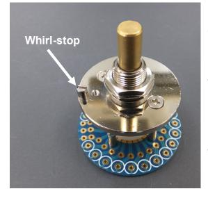
The position of the whirl-stop can be changed easily by removing with the flat-head screwdriver.
