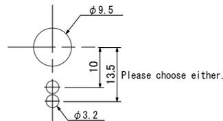
The position of the whirl-stop can be changed easily by removing with the flat-head screwdriver.
