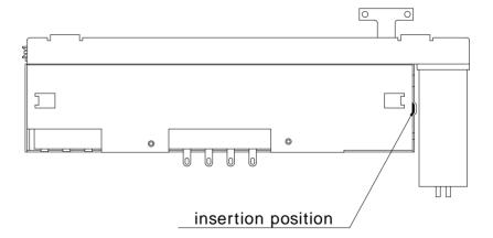
The cover can be removed by inserting a flat-blade screwdriver or a thin metal plate and twisting.
