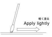
Apply oil to the entire area exposed between the carrier end and the end of the track, about 5 laps.
